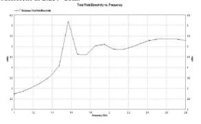
Fig: 5. Directivity vs. Frequency
